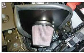
16. Install the K&N<sup>®</sup> air filter onto the filter adapter and secure with the provided hose clamp. NOTE: Drycharger<sup>®</sup> air filter wrap; part # RU-5147DK is available to purchase separately. To learn more about Drycharger<sup>®</sup> filter wraps or look up color availability please visit http://www.knfilters.com<sup>®</sup>.
