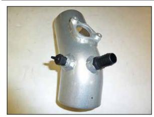
7. Install the provided vent fittings into the K&N<sup>®</sup> intake tube as shown.
