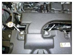
2. Remove the two bolts that secure the fresh air intake duct and then remove the duct from the vehicle.
