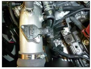
19. Reconnect the mass air sensor electrical connection.
