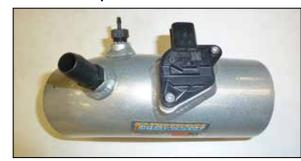
8. Remove the mass air sensor from the factory housing and install it into the K&N<sup>®</sup> intake tube and secure with the provided hardware.
