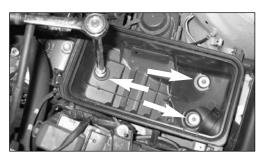
7. Loosen and remove the three bolts that secure the air box base to the vehicle as shown.
