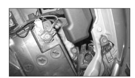
10. Loosen and remove the bolt that secures the air inlet duct to the inner fender as shown.
