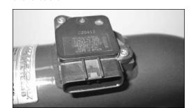
16. Install the MAS into the intake tube using the provided hardware.
