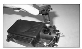
14. Remove the screws from the MAS, then, remove the MAS from the air box as shown.
