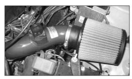
22. Install the Filtercharger onto the Typhoon tube and secure with the provided hose clamp as shown.
