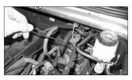
25. Secure the throttle cable to the brake line using the cable tie supplied. Do not fully tighten the cable tie, allow a little slack for the throttle cable!
