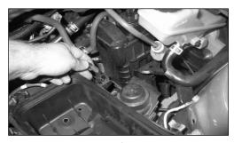
8. Unclip the wire harness from the air box base as
