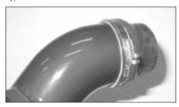
18. Fit the stepped silicone sleeve on the tube using the original hose clamp removed earlier.
