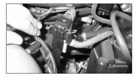
21. Slide the PWM vacuum switching valve onto the "L" bracket as shown.
