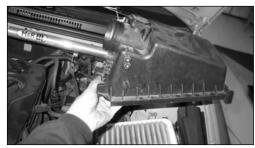
6. Remove the air box lid from the vehicle as shown.
