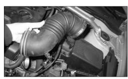
4. Remove the intake tube from the trottle body and the air box. The hose clamps are being used later
