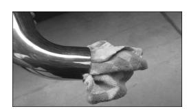
15. Clean the inside of the tube out with water and a towel as shown.
