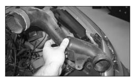
11. Remove the air inlet duct from the vehicle as shown
