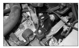
13.Fit the "C" bracket to the rubber mounted stud using a waved washer and nylock nut supplied, but do not tighten completely.
