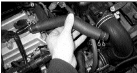
5. Unclip and remove the breather hose from the vehicle.
