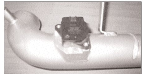
16. Carefully install the MAS into the intake tube using the two M4 Allen head bolts supplied.
