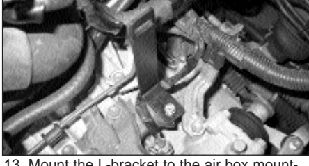
13. Mount the L-bracket to the air box mounting point using the M6 Allen head bolt and wave washer supplied.
