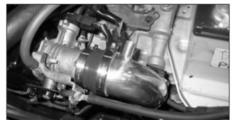
17. Fit the intake tube into the silicone hose using the hose clamp supplied. Do not fully tighten yet!
