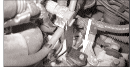
14. Fit the purge valve onto the L-bracket.
