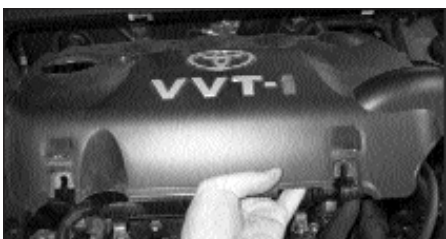
4. Undo the four bolts and remove the engine cover from the vehicle.
