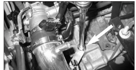
18. Secure the bracket to the threaded hole in the transmission housing using the M10 bolt and wave washer supplied.
