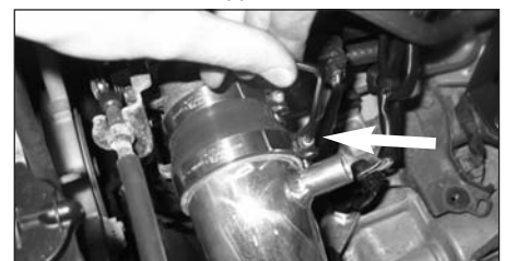
19. Tighten the hose clamp to secure the tube into the silicone hose.
