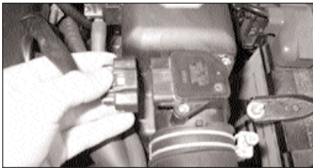
2. Unclip the electrical plug from the Mass Air Sensor (MAS).
