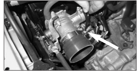
15. Fit the silicone hose onto the throttle body & tighten using the hose clamp supplied.
