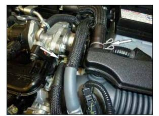
3. Release the spring clamp that secures the PCV hose and then disconnect the PCV hose from the plenum. Loosen the hose clamp that secures intake tube to the throttle body.
