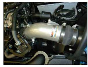
18. Install the intake tube into the couplers, adjust for best fit and then secure with the provided clamps.
