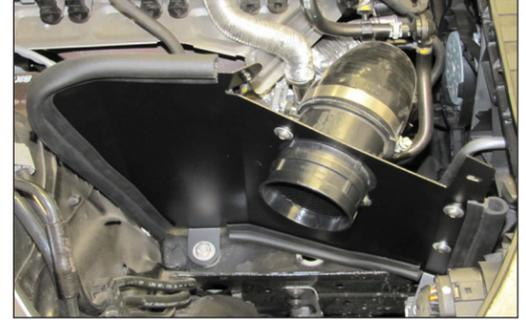
20. Set the heat shield assembly into position on the inner fender while installing the silicone hose onto the turbo inlet. Secure the heat shield with the provided hardware and secure the silicone hose with the provided hose clamps.
