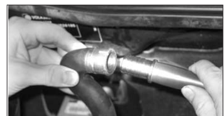
15. Fit the breather hose extension to the original breather hose using the stepped adaptor.
