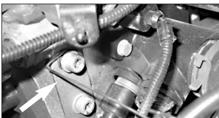
10. Fit the longer hook around the clutch cable and secure it to the engine using the original bolt.
