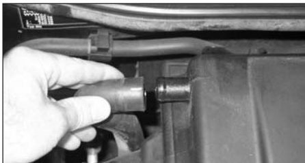
3. Carefully remove the rubber breather hose from the side of the air box.
