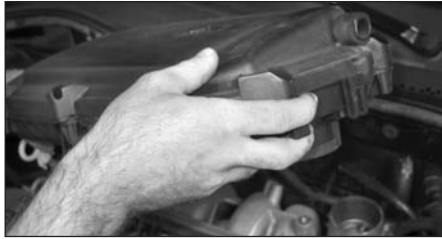
8. Carefully remove the air box assembly from the vehicle.
