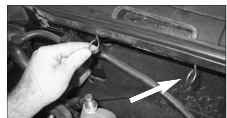
16. Fit the two small hooks under the bulkhead edge trim.
