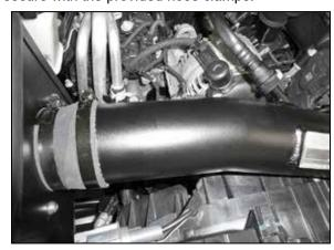
13. Connect the crank case vent line to the K&N® intake tube.
