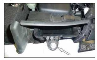
4. Remove the bolt shown that secures the fresh air intake duct to the fender, then lift and remove the complete intake system from the vehicle.
