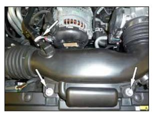
3. Remove the two bolts shown that secure the intake tube to the core support. Push the white locking for the crank case vent line down and then disconnect the crank case vent line from the intake tube.
