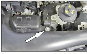
5. Remove the bolt shown securing the intake snorkel to the bracket.
