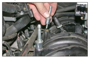
8. On vehicles with the heater hose and wiring harness attached to the air box studs, place a spacer under the two right side air box studs and reinstall the studs into the original location.
