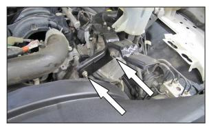
10. Remove the two nuts securing the intake snorkel bracket, then remove the bracket and reinstall the bottom nut.
