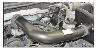
20. Install the K&N® intake tube into the 90° elbow hose and then into the hump hose, align for best fit and then secure with the provided hose clamp. NOTE: On vehicles equipped a Brake Booster/ EVAP vent line, it will be necessary to align the vent line to the tube and mark the tube to be drilled. Remove the tube and drill a 5/8"id hole in the marked location and install the provided grommet, be sure to remove any burrs and
