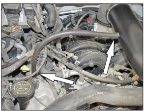
22. Install the provided crank case vent hose onto the vent port on the K&N® intake tube and then onto the vent on the valve cover.
