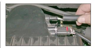
4. On vehicles equipped with a Brake Booster/ EVAP vent line, disconnect the vent line from the air box.
