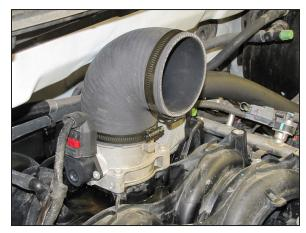
16. Install the provided 90° hose onto the throttle body and secure with the provided hose clamp.
