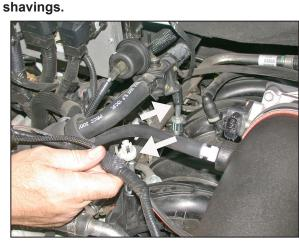
21. Reattach the heater hose and wiring harness to the studs installed in the previous step.
