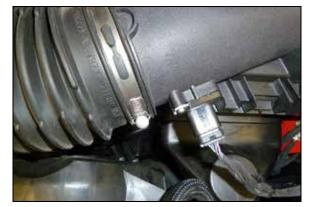
4. Disconnect the mass air sensor electrical connection.
