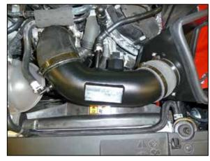
16. Install the intake tube into the coupler at the throttle body and onto the coupler at the filter adapter, adjust the tube for best fit and then secure the tube to the coupling hoses with the provided hose clamp. Connect the EVAP and crank case vent lines to the fittings installed into the K&N® intake tube.
