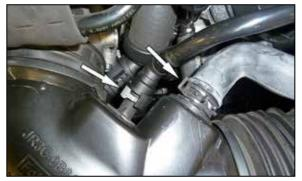
5. Disconnect the vent lines and sound tube attached to the intake tube. Loosen the hose clamps that secure the intake tube to the air filter housing and throttle body and then remove the intake tube from the vehicle.
