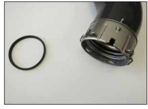
7. Carefully remove the factory O-Ring from the quick connect fitting. **NOTE: Be sure to note the direction of the lip on the seal.**
