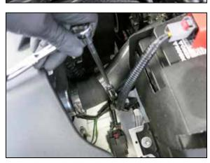
15. Connect the angle coupler onto the K&N inter cooler quick connect fitting and slide the clamps into position.
