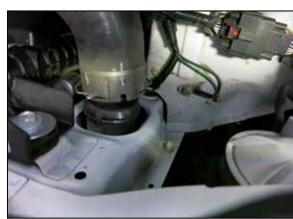
5. Disconnect the factory charge pipe from the throttle body and inter cooler.
