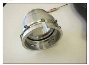
9. Install the factory O-Ring and retaining clip into the provided quick connect fitting, NOTE: Be sure to install the O-Ring in the correct direction for proper sealing. The lip should be towards the inter cooler just how it was in the factory fitting.
