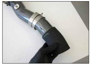
13. Install the clamps and angled coupler onto the K&N charge tube.
