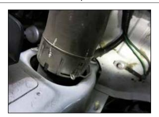
4. Release the charge pipe to intercooler quick connect fitting clip and lock it into the unlock position as shown.
