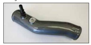
11. Using pipe sealant on the thread, install the quick connect vent fitting and 1/8npt pipe plug into the K&N charge tube.
