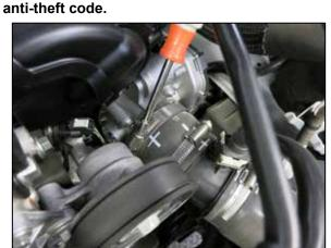
2. Loosen the hose clamp the secures the factory charge pipe coupler to the throttle body.
