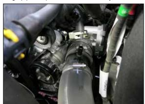
3. Release the white locking clip that secures the vent line quick connect fitting to the factory charge pipe and then disconnect the vent line from the charge pipe.
