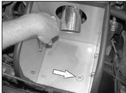
30. Install the remaining hardware, adjust the heat shield for best fit and clearance; tighten all hardware as shown.
