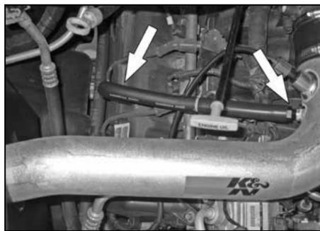
41d. On 2008 and later model year vehicles, install the crank case vent hose assembly onto the valve cover and intake tube as shown.
