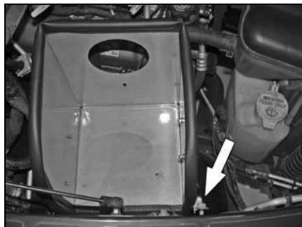
19. Install the heat shield assembly onto the rubber mounted studs and line up the "L" bracket with the threaded hole from step 12 and secure with the stock bolt as shown.
