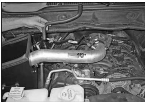
41a. On 2008 and later model year vehicles, remove the crank case vent hose from the passenger side valve cover as shown.
