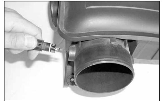
23. On models that come equipped with temp sensors, remove the air temp sensor from the resonator as shown.
