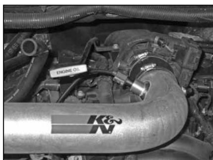
33b. Connect the open end of the inlet air temperature sensor extension harness into the inlet air temperature sensor as shown.
