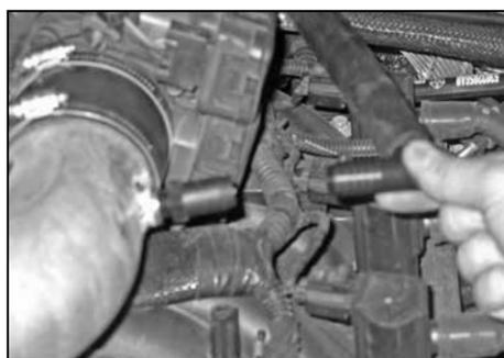
31. On vehicles with the crank case vent hose connected to the "T" on the drivers side of the engine, install the 90° vent fitting into the stock crank case hose as shown.
