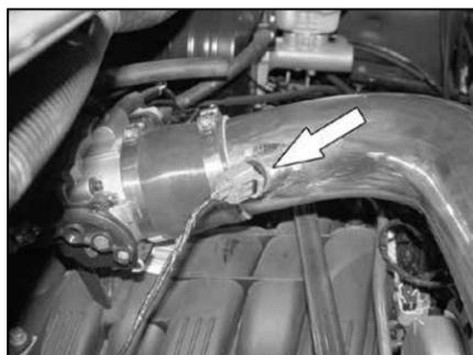
33. On 2002-2007 model year vehicles, reconnect the inlet air temperature sensor electrical connection as shown.
