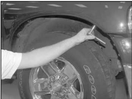
11. Reinstall the inner fender removed in step #9. **NOTE: Two of the retaining bolts will not be used.**
