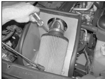
42. Install the air filter and secure with the provided hose clamp as shown.
