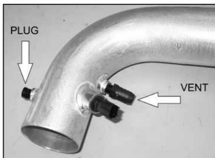
25b. On 2008 and later model year vehicles, install the 1/4"npt vent fitting and plug as shown.
