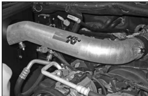
28. Install the K&N® intake tube into the silicone hose at the throttle body and align the mounting bracket with the heat shield. Secure the intake tube with the hose clamp and hardware provided.
