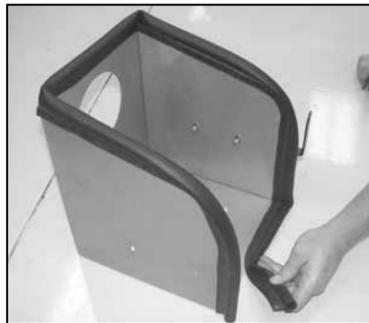
18. Install the provided edge trim onto the heat shield and trim to fit.
