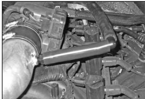
32. Install the provided silicone hose onto the 90° vent, then connect the other end of the silicone hose onto the vent attached to the K&N® intake tube.
