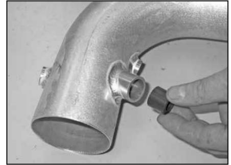
22. On vehicles equipped with an air temperature sensor, install the provided silicone hose into the vent on the K&N® intake tube as shown.
