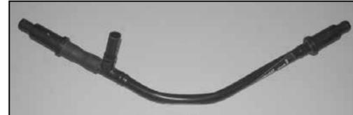
36. Rotate the long side of the vent tube assembly 180° as shown.
