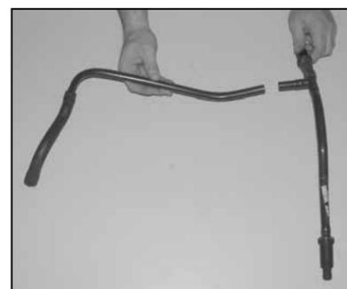
35. Cut the crank case vent tube 1" from the "T" fitting as shown.
