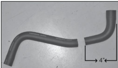
41b. On 2008 and later model year vehicles, cut the factory crank case vent hose 4" from the end as shown.
