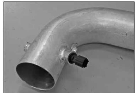
25. On vehicles equipped with an air temperature sensor, install the air temperature sensor into the silicone hose as shown.
