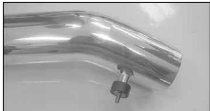
26. Install the rubber mounted stud into the threaded boss on the K&N® intake tube as shown.
