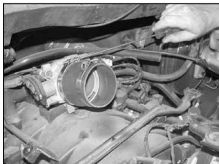
20. Install the silicone hose and hose clamps onto the throttle body and tighten as shown.
