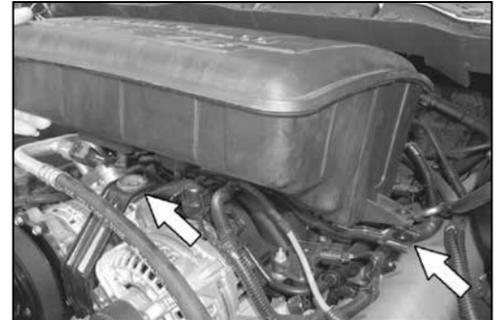
6. Pull up firmly to release the resonator from the engine.
