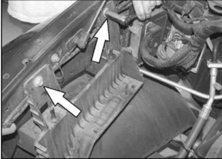
10. Remove the air cleaner support bracket, that is secured by the two bolts on the upper fender and two bolts on the lower fender.
