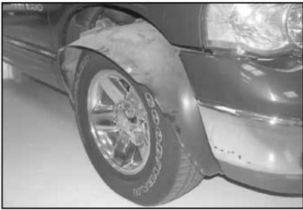
9. Loosen and remove the eight bolts that secure the inner fender valance; lower the valance down as shown.
