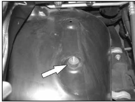
15. Install the provided rubber mounted stud into the existing hole on the inner fender and secure from underneath the inner fender with the provided rubber washer, fender washer and nylock nut as shown.
