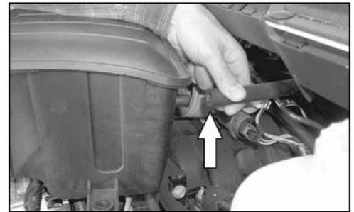
7. On 2002-2007 model year vehicles, disconnect the crank case vent hose from resonator as shown, then remove resonator from vehicle.
