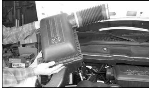
3. Lift up firmly to release the air box from mounting studs, then remove completely.
