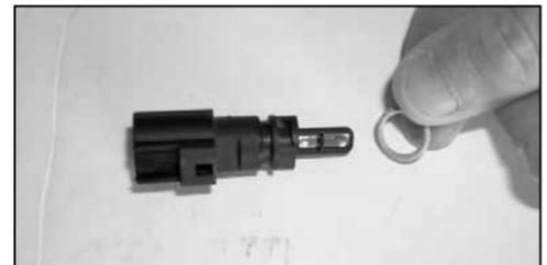
24. Remove the O-ring from the air temp. sensor as shown.
