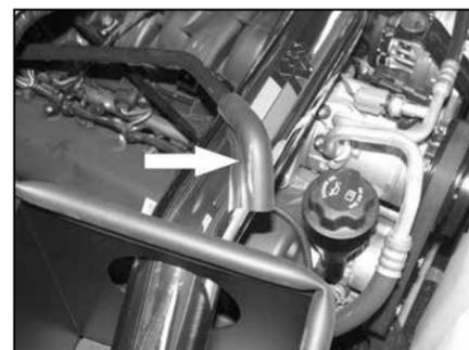
39. On models where the crank case vent hose is connected to the passenger side valve cover, remove the factory 90° coupling hose from the plastic vent tube.
