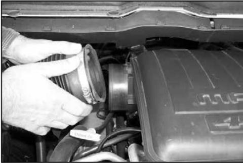
2. Loosen the hose clamp that connects the intake tube to the resonator box then remove the intake tube.
