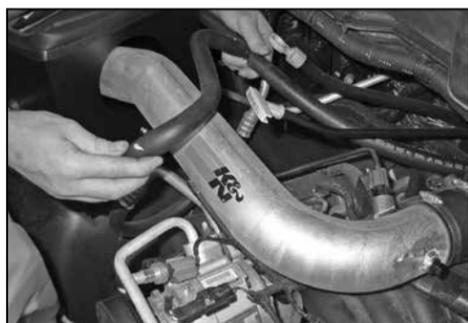
34. On models where the crank case vent hose is connected to the "T" on the passengers side of the engine, remove the complete vent tube assembly from the rubber fittings in each valve cover as shown.
