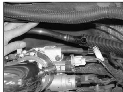
37. Reinstall the vent tube assembly into the rubber fittings in each valve cover so that the "T" fitting is now on the drivers side of the engine facing forward.
