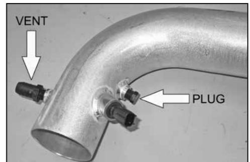
25a. On 2002-2007 model year vehicles, install the 1/4" npt vent fitting and plug as shown.
