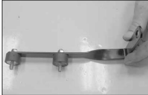
16. Secure the provided rubber mounted studs to the provided "L" twist bracket using the provided hardware as shown.
