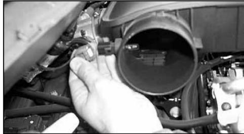
4. On models that come equipped with air temp sensors, unplug the air temp. sensor electrical connection as shown.
