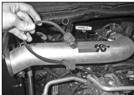
33a. On 2008 and later model year vehicles, connect the provided inlet air temperature sensor extension harness into the factory connection as shown.
