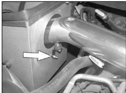
29. Line up the angle bracket with the heat shield and secure with the provided hardware as shown.
