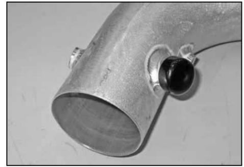
21. On vehicles not equipped with an air temperature sensor, install the provided cap plug and secure with the provided hose clamp.
