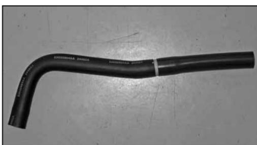
41c. On 2008 and later model year vehicles, install the provided hose mender and crank case vent hose onto the cut factory vent hose as shown.
