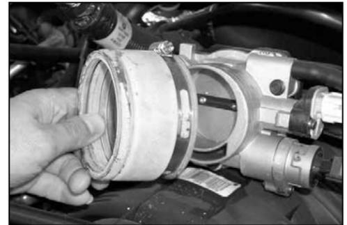
8. On 2002-2007 model year vehicles, loosen the hose clamp that retains the rubber hose to the throttle body and remove as shown.
