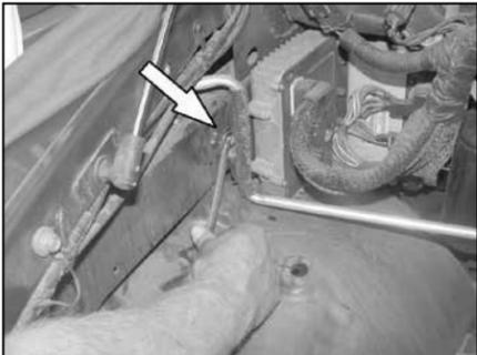
12. Remove the bolt that secures the computer to the inner fender as shown.
