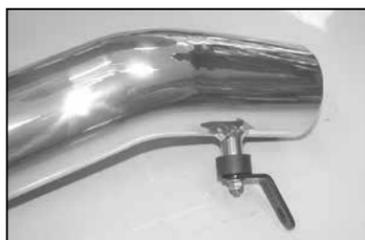
27. Secure the provided small angle bracket to the rubber mounted stud using the provided hardware as shown.
