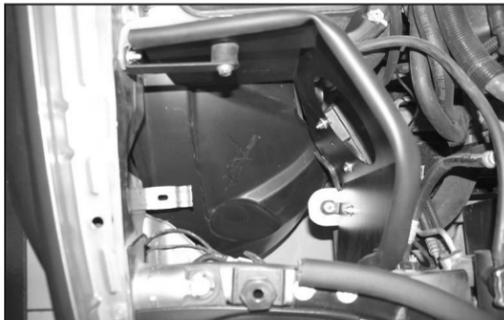
19. Install the heat shield assembly into the vehicle and secure it to the mounting locations with the provided hardware.
