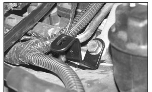
23. Install the tube mounting bracket onto the A/C compressor and secure with the factory mounting bolt removed in step #22.
