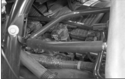
30. Install the supplied silicone hose onto the crankcase vent "T" and connect the other end onto the K&N® intake tube as shown.
