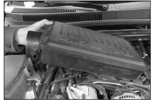
20c. Remove the intake plenum from the vehicle as shown.
