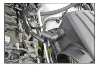
5. Disconnect the crank case vent tube from the elbow attached to the factory air filter housing as shown.
