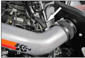
21. Install the provided crank case vent hose onto the fitting installed into the K&N® intake tube and then connect the other end to the factory crank case vent tube.
