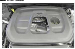
2. Lift up the inspection cover and remove the bolt that secures the decorative engine cover. Then remove the decorative engine cover from the
