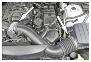
4. Loosen the hose clamps securing the intake tube to the throttle body and air filter housing and then remove the intake tube assembly from the vehicle.
