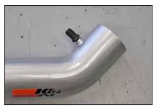
17. Install the provided vent fitting into the K&N® intake tube as shown.
