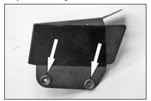
9. Install the two mounting grommets from the previous step into the  $K\&N^{\tiny\textcircled{\tiny 0}}$  heat shield as shown.
