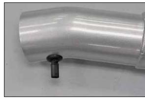
16. Install the provided grommet into the K&N® intake tube then remove the O-Ring from the inlet air temperature sensor and then install the sensor into the grommet install into the K&N® intake tube. NOTE: The inlet air temperature sensor is very fragile, use care while handling the sensor.
