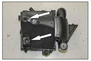
8. Remove two of the mounting grommets from the factory air filter housing.
