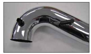
11. Install the inlet air temperature sensor into the K&N® intake tube using the provided grommet. Install the 90° NPT fitting onto the K&N® intake tube as shown.
