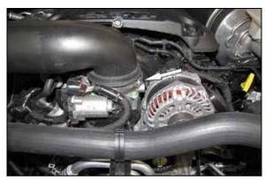
3. Loosen the hose clamp at the throttle body and then lift the complete intake system out of the vehicle.
