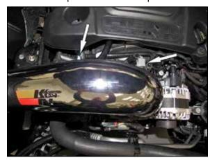
13. Connect the crank case vent line and inlet air temperature sensor electrical connection.
