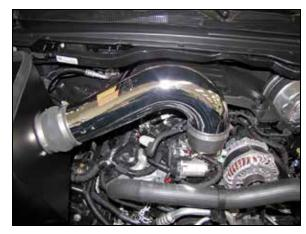
12. Install the K&N® intake tube into the coupler at the heat shield and then into the coupler on the throttle body, adjust the tube for best fit and then secure with the provided hose clamps.
