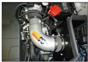
16. Install the K&N® intake tube into the coupler and adjust for best fit, then secure with the provided hose clamps.
