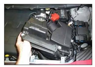
7. Lift the air filter housing assembly to dislodge it from the mounting grommets and then remove the housing from the vehicle.
