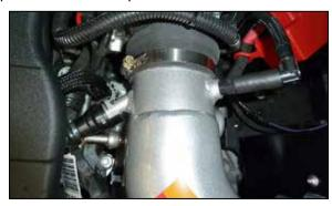
17. Connect the CCV fitting to the fitting on the intake tube and connect the EVAP line to the hose connect to the K&N® intake tube.
