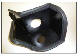
9. Install the provided edge trim onto the heat shield as shown.
