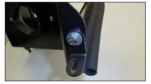
12. Install the provided mounting bracket onto the heat shield using the provided hardware.
