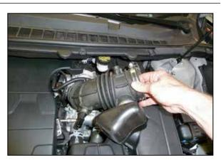
5. Remove the intake tube from the vehicle. NOTE: K&N Engineering, Inc., recommends that customers do not discard factory air intake.
