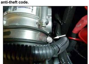
2. Loosen the hose clamp that secures the intake tube to the throttle body.
