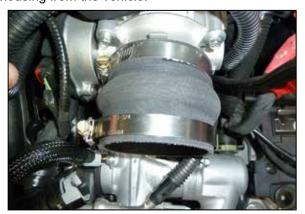
8. Install the provided hump coupler (08171) onto the throttle body and secure with the provided hose clamp.
