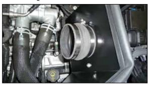
14. Install the provided hump coupler (08699) onto the filter adapter and secure with the provided hose clamp.
