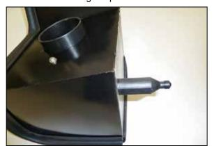
11. Install the mounting stud onto the heat shield using the provided hardware.
