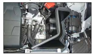
13. Install the heat shield assembly so the mounting stud inserts into the factory mounting grommet and then secure with the factory fresh air duct mounting bolts.
