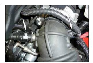
3. Disconnect the crank case vent hose from the factory intake tube and unhook the vent line that is attached to the tube.
