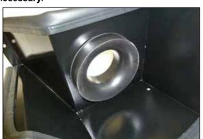
10. Install the provided filter adapter into the heat shield as shown using the provided hardware.
