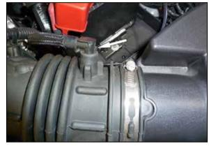
4. Disconnect the EVAP vent line and fitting from the intake tube. Loosen the hose clamp securing the intake tube to the air filter housing.
