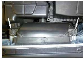
6. Remove the two bolts securing the fresh air intake duct to the core support.
