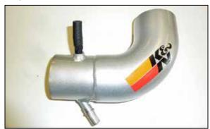
15. Install the provided vent fitting and EVAP hose onto the  $K\&N^{\mbox{\scriptsize 0}}$  intake tube as shown.
