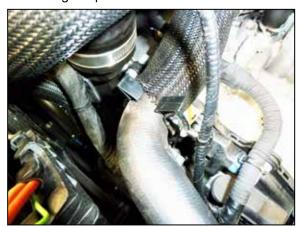
9. Move and rotate the IAT harness clamp to the position as shown.
