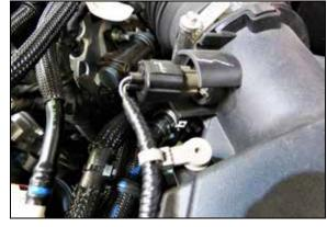
4. Disconnect the AIT sensor electrical connection and unhook the wiring harness from the air filter housing.
