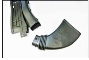
3. Separate the air filter housing end from the fresh air duct.
