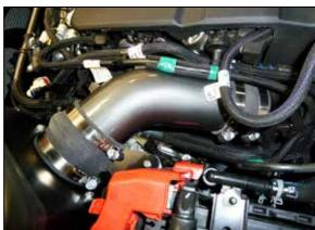
15. Install the intake tube into the couplers and adjust for best fit, then secure with the provided hose clamps.
