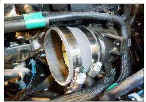
10. Install the provided coupler onto the turbo inlet pipe and secure with the provided hose clamp.
