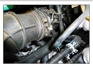
5. Loosen the hose clamp that secures the factory intake tube to the turbo inlet. Disconnect the hose from the inlet and then lift out the complete intake system.
