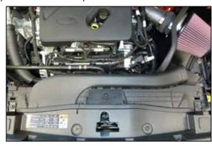
18. Reinstall the fresh air intake duct and secure with the factory push pins.
