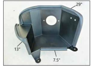
6. Cut the provided edge trim into sections of 7.5", 13" and 29" long. Install the edge trim onto the heat shield as shown.
