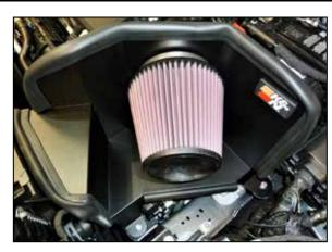
17. Install the K&N air filter and secure with the provided hose clamp.
