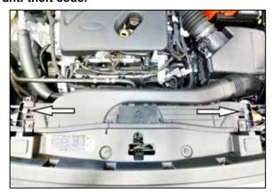
2. Lift the center of the locking pins that secure the fresh air duct and then remove the pins. lift the fresh air duct and disconnect it from the air filter housing and remove it from the vehicle.
