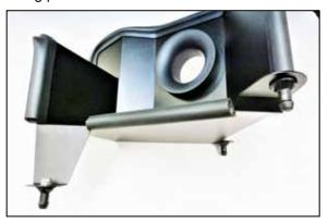
8. Install the three mounting posts onto the heat shield using the provided hardware.
