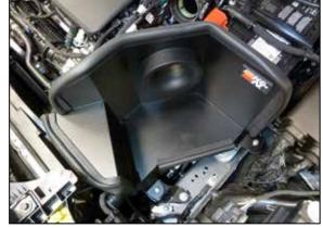
11. Install the heat shield assembly into the vehicle so the mounting studs insert into the factory air filter housing mounting grommets.
