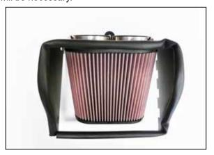
6. Install the K&N air filter into the heat shield.
