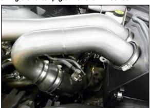
13. Install the front K&N intake tube into the filter and then into the driver side turbo inlet tube, adjust for best fit and secure with the provided hose clamps.
