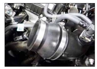
10. Install the provided step coupler onto the driver side turbo inlet tube and secure with the provided hose clamp.
