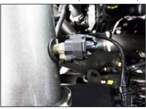
12. Connect the IAT electrical connection. NOTE: It may be necessary to use the provided extension harness due to some vehicles having a shorter pigtail for the IAT sensor.
