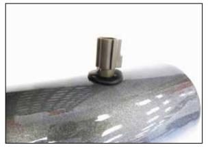
8. Remove the AIT sensor from the factory intake tube. Remove the O-ring from the sensor and then install it into the K&N intake tube with the provided grommet. NOTE: The IAT sensor is fragile, use caution while handling the sensor to prevent damage.
