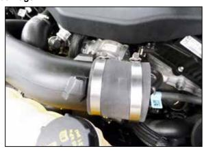
9. Install the provided straight coupler onto the passenger side turbo inlet tube and secure with the provided hose clamp.
