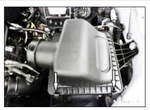
4. Release the clips that secure the factory air filter upper housing and remove the housing and factory air filter from the vehicle.
