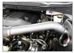
11. Install the rear K&N intake tube into the air filter and passenger side turbo inlet tube, adjust for best fit and then secure with the provided hose clamps.
