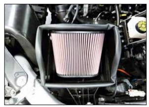
7. Place the heat shield assembly onto the factory lower air filter housing so that the tabs seat into the housing. Secure the heat shield with the factory retaining clips.
