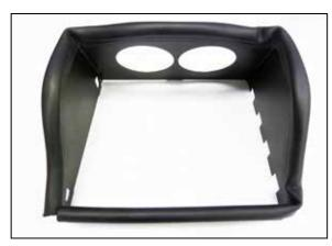
5. Install the provided edge trim onto the K&N heat shield as shown. Some trimming of the edge trim will be necessary.
