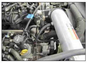
18. Install the provided crank case vent hose onto the fitting installed into the K&N® intake tube and then onto the valve cover port. Secure the hose to the valve cover port with the provided hose clamp.
