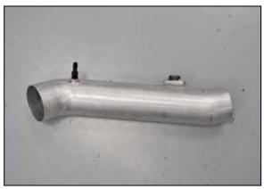
14. Install the provided vent fitting into the K&N<sup>®</sup> intake tube as shown.
