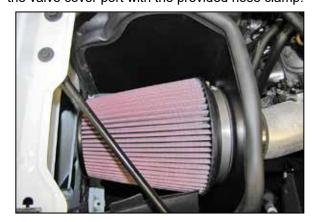
19. Install the K&N $^{\!0}$  air filter and secure with the provided hose clamp.
