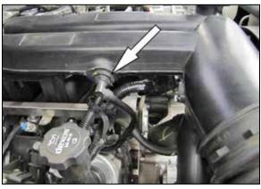
4. Disconnect he crank case vent hose from the intake tube plenum.
