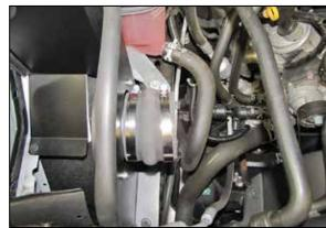
15. Install the provided coupling hose (08699) onto the filter adapter and secure with the provided hose clamp.
