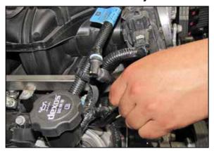
7. Release the locking ring and then disconnect the crank case vent tube from the valve cover vent port.
