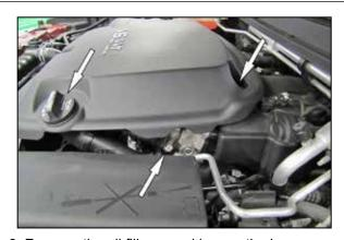
3. Remove the oil fill cap and loosen the hose clamp securing the intake hose to the throttle body. Remove the bolt securing the intake plenum to the engine.
