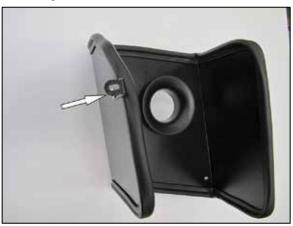
9. Install the provided heat shield mounting bracket (07805) onto the heat shield using the provided hardware and spacer.
