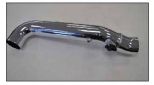
13. Remove the mass air sensor from the factory air filter housing and install the sensor into the K&N® intake tube using the provided hardware.
