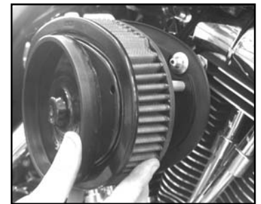
17. Install the air filter element onto the base plate.
