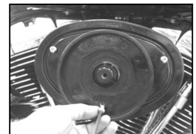
18. Install the three provided button socket bolts. Item G on the parts list. Do not completely tighten.
