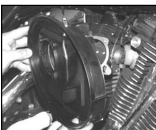
5. Remove the stock back plate. Note: Retain the stock air cleaner gasket, it will be reinstalled in a later step.
