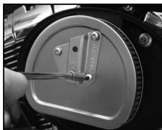
2. Remove the three torx bolts.
