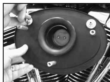
13. Install the back plate and thread the stock breather bolts into the breather bolt extensions. Do not tighten at this time. Note: For 2006-2007 fuel injected models, install a washer in between the back plate and each of the provided breather bolt extensions. Thread the stock breather bolts into the breather bolt extensions. There should be a washer on each side of the provided breather bolt.
