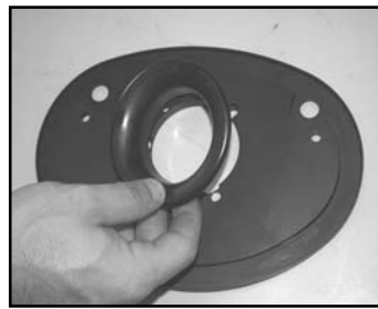
6. Install the velocity stack onto the supplied back plate.
