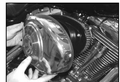
19. Check the perimeter of the back plate to ensure the air filter element is completely seated.
