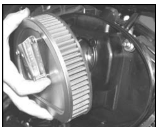
3. Remove the stock air filter element.
