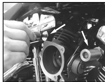
11. Install the provided breather bolt extensions into the stock breather bolt location.
