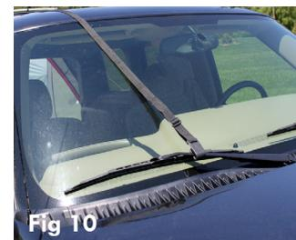
**10-**Adjust the baffle inside the top edge of the upper sleeve to keep water, wind, and bugs out.
