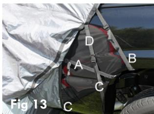
15-Run the lower strap (C) under the rear wheel well and route it up to snap onto the upper strap (D) (Fig 13).
