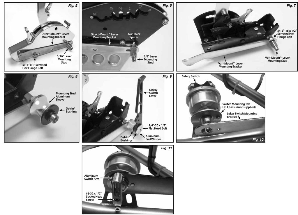
Interior Battery Disconnect Lever Kit Installation Instructions
