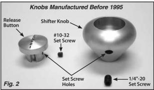
Step 2: (Continued) For shifter knobs manufactured before 1995, set the release button into the shifter knob, and screw the shifter knob onto the lever. When the release button gets close to being flush with the top of the knob, hold the release button so that the shift pattern letters are in the proper position. Continue to thread the shifter knob onto the shifter lever until the release button is flush with the top of the knob.
