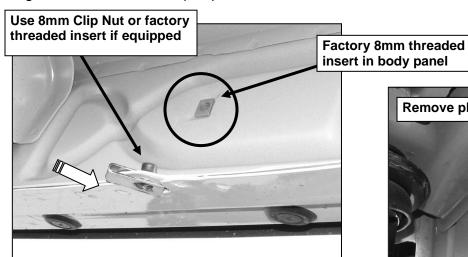
(Fig 1) Example of mounting location with factory threaded hole
