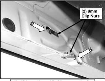
(Fig 3) Insert 8mm Clip Nut as required
