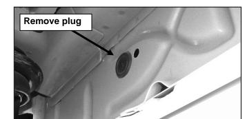
(Fig 2) Example of mounting location without factory threaded hole in rocker panel
