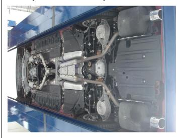
**Step 2.** Install the new system by loosely attaching the new X-Pipe Assembly to the catalytic converter using the OEM hardware and by locating the welded hanger to the rubber isolator. Leave all clamps and fasteners loose for final adjustment of complete system.
