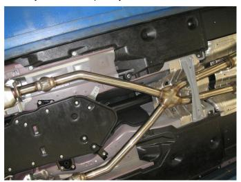
**Step 3.** Loosely attach the two Resonator Assemblies using the supplied 2.50" clamps and engaging the welded hangers to the rubber isolators..
