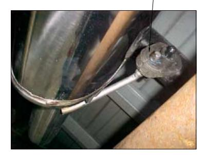
**Step 3:** With all components mounted loosely, adjust the system for overall aesthetics and clearance of frame & bodywork. (MAGNAFLOW recommends at least 1/2" of clearance between the exhaust system and any body panels to prevent heat-related body damage or fire.)
