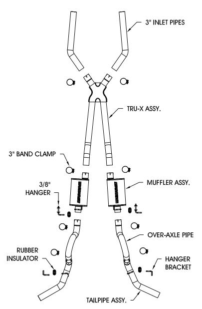
**Note**: This system is designed to work with OEM-style exhaust manifolds, or tubular headers. Due to the various applications possible, some modification and welding is required for a proper fit and finish.
