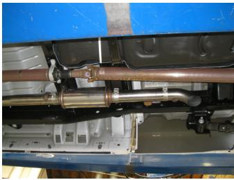
**Step 4.** Install the Muffler, Tail Pipe Assembly and Extension Pipe Assembly (if needed) using the supplied 3.50" clamps. Locate the welded hangers to the OEM rubber insulators.
