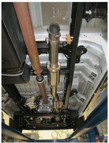
**Step 5.** Once a final position has been chosen for the new exhaust system, evenly tighten all clamps from front to rear using the torque specifications on page one of the instructions. Inspect all fasteners after 25-50 miles of operation and re-tighten if necessary.
