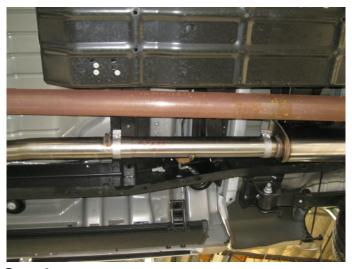
**Step 3.** Install the Muffler using the supplied 3.50" clamp. Use the supplied 16.00" Extension Pipe between the Muffler and the Tail Pipe Assembly if your truck uses the Crew Cab Long Bed or the Extended Cab Short Bed configuration. If your truck has a Crew Cab with the Short Bed the 16.00" Extension Pipe is not used.
