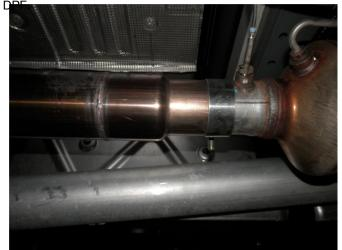
**Step 2.** Begin installation of your new MAGNAFLOW system by loosely attaching the Inlet Pipe Assembly to the DPF outlet pipe you have just cut using the supplied 2.75" clamp. Engage the welded hangers to the rubber insulators. Reinstall the secondary O2 sensor.
