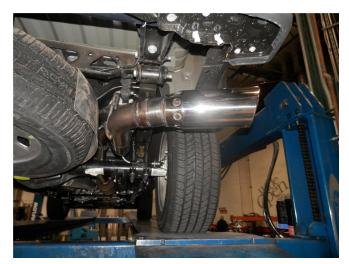
**Step 3.** Loosely attach the Tail Pipe Assembly using a similar fashion. Keep all fasteners loose for final adjustment.
