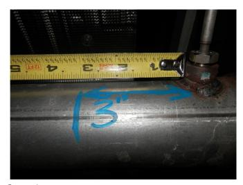
**Step 1.** Begin removal by removing the secondary O2 sensor at the over axle pipe of the OEM system. Next, cut the OEM inlet pipe 3.00" rearward of the O2 sensor behind the
