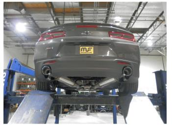
**Step 4.** Once a final position has been chosen for the new exhaust system, evenly tighten all clamps from front to rear using the torque specifications on page one of the instructions. Replace the shield and cross brace. Inspect all fasteners after 25-50 miles of operation and re-tighten if necessary.
