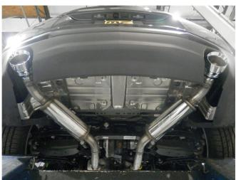
**Step 3.** Begin installation by loosely attaching both drivers side and passengers side Muffler Assemlies to the outlet of the cut pipes using the supplied clamps and fitting the hanger into the rubber insulator. Leave all clamps loose until final adjustment
