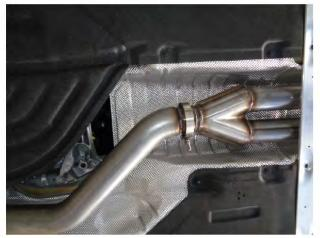
**Step 3.** MagnaFlow supplies this kit with multiple build options giving the ability to use different inlet pipe diameters and delete the mufflers depending on preference.
