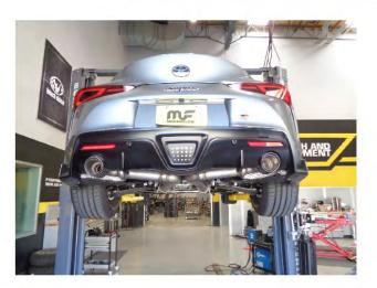
**Step 6.** Once a final position has been chosen for the new exhaust system, evenly tighten all clamps and fasteners, from front to rear, using the torque specifications on page one of the instructions. Inspect all fasteners after 25-50 miles of operation and re-tighten if necessary.
