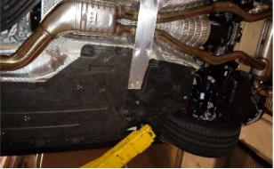
**Step 1.** To remove the OEM system first unplug the electrical connector at the exhaust valve located on the passenger side Tail Pipe. Begin by removing the cross brace then unbolt the mounting bracket and loosen the clamp at the exhaust inlet. Remove all welded hangers from the rubber insulators and remove the exhaust. Do not damage the fasteners or rubber insulators as they will be used to install the new MagnaFlow system.
