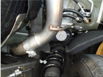
**Step 6.** Next loosely attach the Mid Pipe Assembly to the Muffler Assembly using the supplied clamp. Engage the welded hanger to the rubber insulator.
