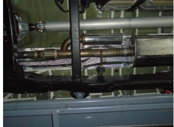
**Step 4.** To begin, fasten the Inlet Resonator Assembly to the outlet of the OE system using the OE clamp and by fitting the welded hanger to the rubber insulator (Leave all clamps and fasteners loose for final adjustment of the complete system.)
