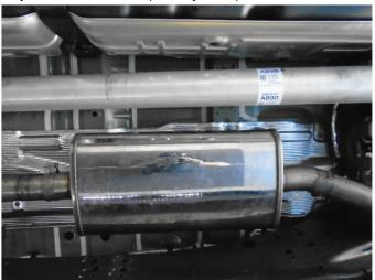
**Step 5.** Attach the Muffler Assembly to the Inlet Resonator Assembly with a supplied 3.00" clamp. Engage the welded hanger to the rubber insulator.
