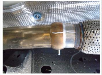
**Step 2.** Unfasten the clamp attaching the OE inlet pipe assembly to the catalytic converter. Do not damage or discard the inlet pipe clamp or rubber insulators as they will be re-used to mount the new system.
