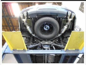
**Step 1.** To remove the OE exhaust system you will need to remove the spare tire, heat shield and sway bar.
