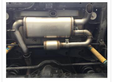
Step 2. Next, slide the MagnaFlow axle-back into the OE over-axle pipe and loosely clamp to hold in place. Then slide the hangers into the factory rubber insulaters. Next attach the NDT resonator and clamp in place.
