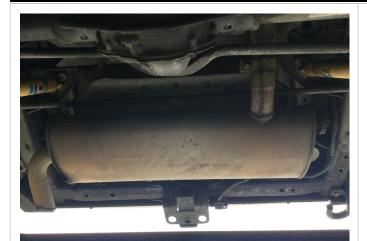
Step 1. Remove the OEM system by loosening the over-axle TORCA clamp. Then disconnect the OE rubber hangers and remove the OE muffler.
