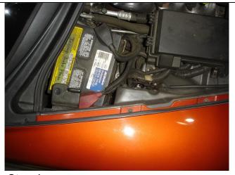
**Step 1.** Before removing the OEM manifold system, first disconnect the battery using a 10mm socket. Remove the engine covers by gently pulling to disengage it from the rubber grommets.
