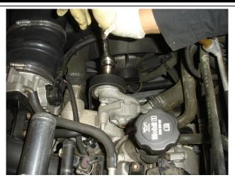
**Step 4.** On the passenger side release the pressure on the drive belt tensioner with a 15mm socket and remove the serpentine belt.
