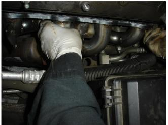
**Step 9.** Reinstall the O2 sensors on your new header assemblies. With the supplied gaskets and header bolts install the header assemblies with a 10mm socket to the manufacturers torque specifications.
