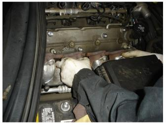
**Step 8.** Unbolt and remove both driver and passenger side manifolds with a 10mm socket. Remove the O2 sensor from the manifolds using a 7/8" wrench.
