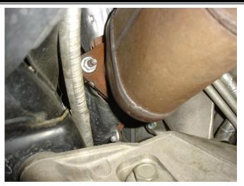
**Step 7.** Using a 15mm socket unbolt both catalytic converters from the OEM manifolds.
