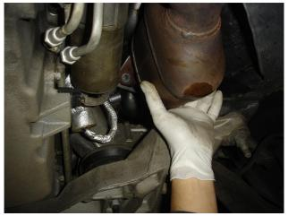
**Step 11.** Align the OEM converters up to the new headers and attach using the supplied nuts and bolts. Tighten the bolts to the manufacturers torque specifications. After all OEM parts have been reinstalled reconnect the battery.
