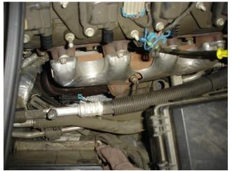
**Step 2.** Disconnect both O2 sensors from the OEM manifolds.
