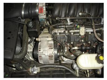
**Step 5.** Using a 15mm socket unbolt the alternator and remove. After alternator has been removed repeat passenger side process to remove the coil pack bracket.
