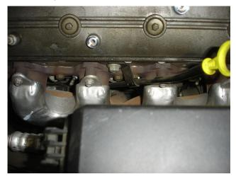
**Step 6.** Using a 15mm socket remove the dipstick assembly.
