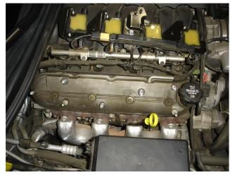
**Step 3.** Remove all spark plug wires from the coils and the plugs, and then set aside. On the passenger side unbolt the coil pack bracket using a 10mm socket and gently flip the assembly towards the upper part of the motor.
