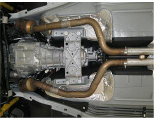
**Step 4.** Unbolt the driver side and passenger side catalytic converter assemblies from the manifold using a 10mm socket and remove. Unbolt the clamps on the back of both converter assemblies and then loosen. Both converter assemblies can now be removed.
