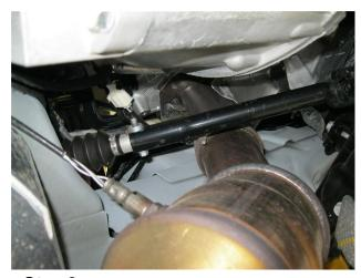
**Step 2.** Using a 7/8" wrench remove the O2 sensors located on the manifold and catalytic converter assemblies.
