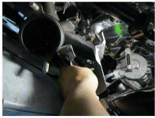
**Step 6.** Unbolt and remove the heat shields from both manifolds using a 10mm socket.
