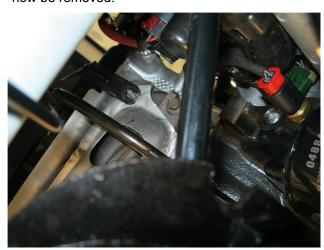
**Step 5.** Unbolt the dipstick assembly on the passenger side using a 10mm socket and remove.
