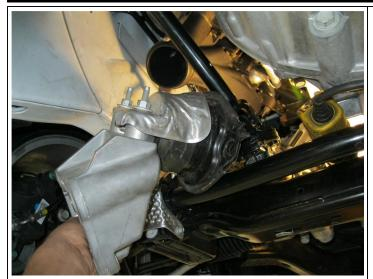
**Step 7.** Unbolt the driver side motor mount using a 15mm socket and then remove.
