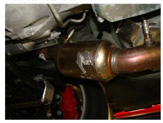
**Step 3.** On the passenger side using a 13mm socket remove the heat shield surrounding the starter.
