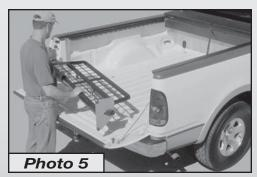
outboard to permit the wheels to enter the Tracks (*Photo 4*). Next, maneuver the Cargo Manager Divider around the back bed posts and rotate the Divider to insert the lead wheel on each side (*Photo 5*). With the lead wheels in place, squeeze the Linkage Control Levers to retract the linkage and rotate the Divider to the vertical position, then align and insert rear wheels. With the wheels in place, press the Track Stop Pins inboard to prevent the wheels from leaving the Tracks.
