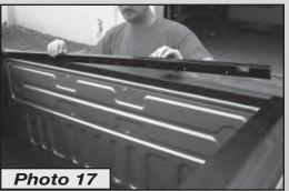
passes through the shim described in Step (A) above. Secure the two remaining holes.
