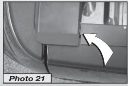
toward the tailgate (Photo 20) so that the Track End Caps contact the inside surface of the tailgate. Make sure the Track End Cap metal blocks contact the Tailgate Extrusion End Caps (Photo 21). Note: If the Tracks are not positioned as shown, the Latch Mechanism will not function correctly.
