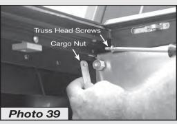
(Photo 39). Tighten these connections securely.
