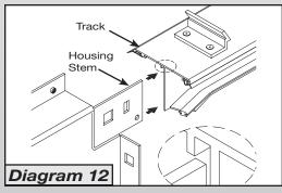
**D** Using 1/4-20 x 1-1/4" countersunk screws, loosely secure the Tracks to the threaded blocks (Photo 13). Do not tighten.
