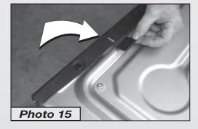
C₌ While holding the Tailgate Extrusion in place, use a #8 x 3/4" self tapping screw
