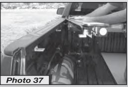
**B** Lower the tailgate and place the driver's side Track onto the bedrail (Photo 37), and key it onto Housing Stem (Diagram 38), being sure that the Handle is properly engaged into the Track.
