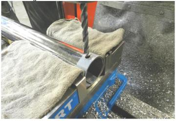
5. Now do the same with the bottom tube using the paper strip labeled 206250 that has the holes centered. The alignment of this tube will not matter because it is the same all around.
