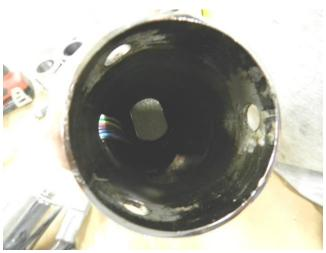
7. Take the electric motor assembly with the adapter already on it and slide it up into the upper bell half of the column. Make sure the coupling is tight on the motor and that the column shaft goes into the coupler a safe distance. Once it is in tighten the set screw through the hole in the column to tighten the coupler on the column shaft and screw the three screws into the unit to hold it together.
