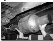
3. Attach the factory catalytic converter to the **Mid Pipe** by placing the gasket
