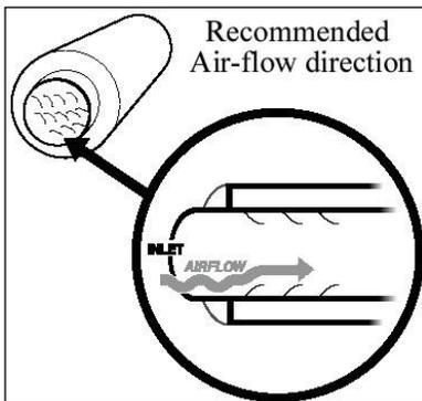
2. Install the **Muffler** over the **Extension Pipe** so that the exhaust will flow smoothly over the louvers. Refer to the illustration on the left.
