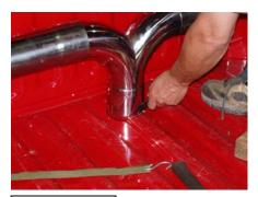
5. Mark the bed floor where the "T" Pipe is resting. MBRPinc. recommends tracing around where the "T" Pipe meets the bed floor. Remove the stacks, "T" Pipe, and Elbows from the bed of the truck. Find the center of the circle traced onto the bed floor, mark and center punch it. Make sure that there is clearance for the Quad Cab Elbow to pass by any frame cross members. See Fig 4.
