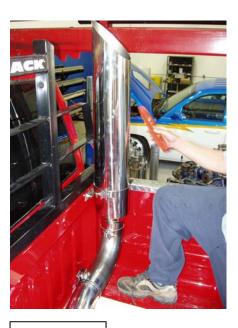
7. Set the "T" Pipe, assembled with the 13" and 37" Elbows at the desired height from the floor of the bed (This will set the height of the stacks). Using spacers to hold the "T" Pipe and both 13" and 37" Elbows at the desired height, loosely attach the stacks to the Stack Mounting Brackets making sure that they are straight. See Figure 6.
