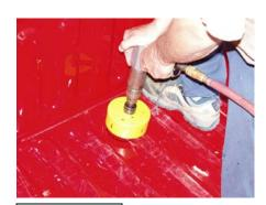
6. Cut a hole through the truck bed providing adequate clearance around the part of the "**T**" **Pipe** that passes through the truck bed. MBRP inc. recommends using a 5" diameter hole saw. It may be required to cut part of a bed floor rail away. **See Figure 5.**
