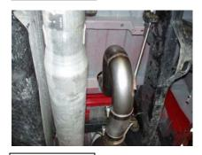
9. Install the assembly from step 8 onto the vehicle by inserting the outlet of the **Quad Cab Elbow** into the inlet of the **T" Pipe.** Install the hanger into the factory rubber isolator. Slide the **Flexpipe** onto the outlet of the DPF. **See Figure 8**.
