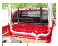
10. Make sure the **Stack Mounting Brackets** are centered on the stacks and tighten the fasteners holding the **Stack Mounting Brackets** to the front of the truck bed. Tighten all **Clamps** to ensure your "Smokers" exhaust system remains properly aligned. **See Figure 9.**
