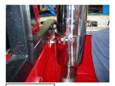
3. Loosely attach the **Stack Mounting Bracket** to the front of the truck bed using the **3/8**" hardware supplied. Set the stack up in the bed and loosely attach it to the **Stack Mounting Bracket**. Make sure the stack is vertical and in the desired position. **See Figure 3**.
