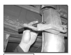
10. Measure from the "**T**" **Pipe** slip joint to the exhaust system that you are connecting to. Mark and cut the shorter side of the **20**" **Elbow** to the required length so that it lines up with the front part of the exhaust system. **See Figure 9**.
