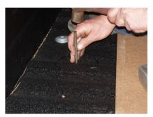
4. Mark the bed floor where the stack is resting. This is where the **Extension Pipe** will pass through the floor. Remove the stack from the bed of the truck. Find the center of the circle traced onto the bed floor, mark and center punch it. Drill the hole using a 5" hole saw. It may be required to cut part of a bed floor rail away. **See Figures 5 and 6.**
