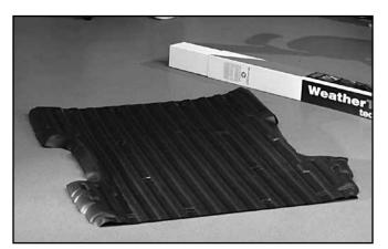
Remove TechLiner<sup>®</sup> from the shipping box and lay it face down on a dry, flat surface\*. Warm sun will help the TechLiner<sup>®</sup> to flatten. DO NOT install if temperature or truck bed itself is below 50° F. \*Take note of the location of the Velcro pads on the bottom of the TechLiner<sup>®</sup>, and prevent pads from becoming dirty or collecting debris.
