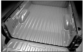
Remove all other bed and tailgate accessories prior to installation. TechLiner<sup>®</sup> is to only be installed in a truck bed that is in original, as-new condition; free of rust, contamination, scratches, previous spray-in bedliners, etc.
