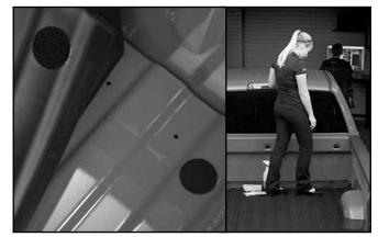
Remove the plastic backing from the Velcro disc and press the TechLiner® back into place. Step on each Velcro disc for a minimum of 15 seconds, this will help the discs adhere.
