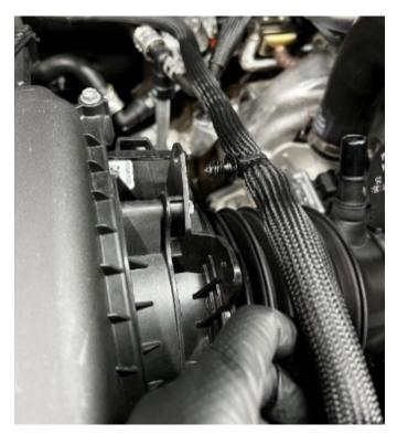
**06.** Pull back the flexible part of the stock intake tube from the plastic section, then lift the airbox assembly straight up to disengage the rubber grommets.
