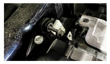
**03.** Loosen the worm gear clamp securing the flexible part of the stock intake tube to the plastic section. Unlock the vacuum line fitting by lifting the tabs up and pushing them back. Next, lift the vacuum line up and out of the way.
