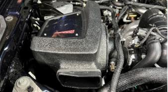
**11.** Reinstall the stock fresh air duct and fasten it with the pop clip. Secure the coolant line tree clip to the Mishimoto airbox as shown.
