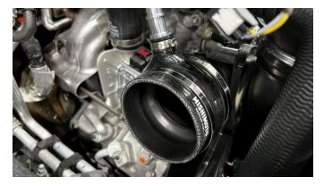
09. Assemble the Mishimoto intake as shown. Fasten the bracket and CNC pegs to the airbox with the provided hardware, then install the rubber grommet and air filter to the rotomold tube. Push the rubber grommet all around until the barb fully engages with the airbox opening.
