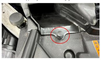
02. Remove the 8mm bolt holding the stock airbox to the fender frame.
