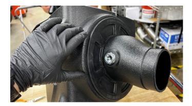
10. Remove the IAT sensor and the rubber grommet with a metal insert from the stock intake, then transfer it to the Mishimoto intake tube and airbox bracket. Next, line up the intake tube with the silicone coupler and lower the Mishimoto intake assembly into the engine bay. Push down on the airbox to engage the metal pegs with the rubber grommets.
