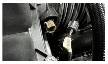
**05.** Disengage the tree clip holding the coolant line from the stock airbox.
