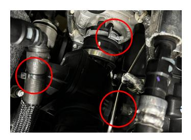
**09.** Remove the charge pipe. Release the tree clip holding the coolant hose to the charge pipe. Loosen the worm gear clamp near the battery. Disconnect the surge valve hose from the driver-side intake hose. Remove 4x 8mm bolts, then release the 2x spring clips to remove the charge pipe from the engine bay.
