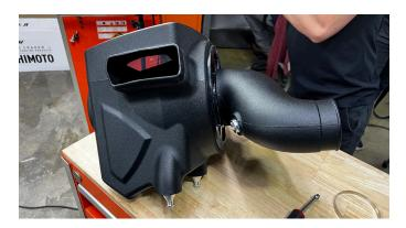
12. Install the Mishimoto airbox and split tube assembly to the stock location and push down on the airbox to engage the bottom pegs. Clip the coolant line tree clip to the side of the airbox as shown.
