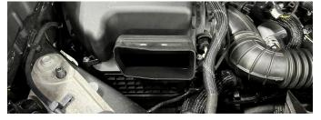
02. Remove 1x bolt holding the airbox to the fender frame.
