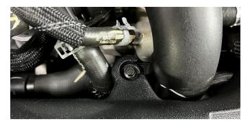
16. Reverse step 9 to reinstall the charge pipe. Use the 2x provided 10mm hex head bolts to fasten the charge pipe to the Mishimoto intake pipe.
