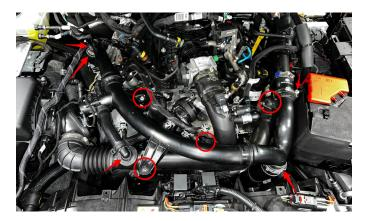
10. Loosen the worm gear clamp, then remove the driver-side intake hose. (Second image on top right)
