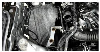
**08.** Remove the passenger side intake hose. Unclip the coolant hose, then remove the bolt securing the intake hose to the engine block.
