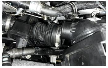
**06.** Unplug the surge valve harness and slide the retainers out from the studs. Move this harness out of the way to remove the airbox.
