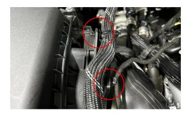
**04.** Unplug the intake air temp sensor and unclip the harness from the airbox.
