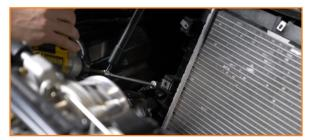
11. Pick the clip from the quick-disconnect attached to the radiator. Then separate the quick-disconnect from the radiator.(1x spring clip)
