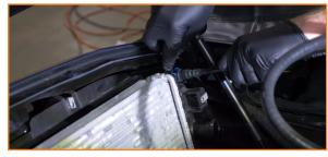
13. Release the AC line. Lift the tab that secures it.
