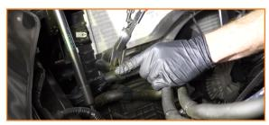
8. Disconnect the electrical connector for the fan shroud and free its wiring harness.
