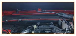
Free the washer fluid line's clip that's secured to the bracket. (1x tree clip)
