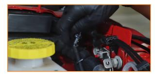
Install the bracket over the two bolts you loosened. (2x 16mm bolts)
