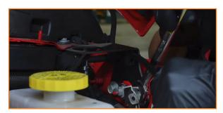
Clip the washer fluid line to the bracket. (1x tree clip)
