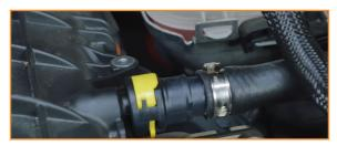
19. Install the open end of the shorter hose to the catch can's OUT port. (1x worm gear clamp)
