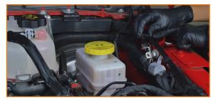
4. Loosen the two bolts on the fender, leaving enough room to fit your bracket. (2x 16mm bolts)
