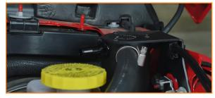
18. Connect the quick-disconnect on the shorter hose to the intake manifold.
