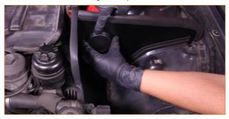
**07.** Install the provided Nyloc nuts over the studs along the frame rail. Install the regular nut and washer over the stud near the fender. (2x 10mm Nyloc nuts, 1x 10mm nut and washer)
